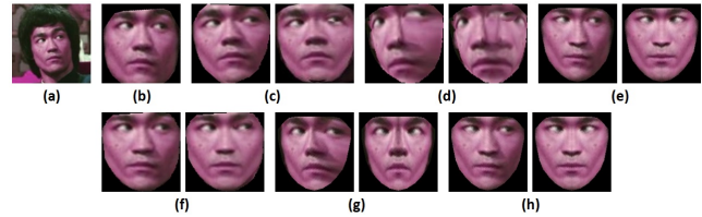
Figure 1: Examples of different pre-processing on a sample image (a) from the CASIA-WebFace dataset [51]: (b) 2D aligned – no frontalization, (c) Zhu and Ramanan [55] & Hassner et al. [15], (d) Kazemi and Sullivan [23] & Hassner et al., (e) CMR & our frontalization method (OFM), (f) CMR & Hassner et al. [15], (g) Zhu and Ramanan [55] & OFM, and (h) Kazemi and Sullivan [23] & OFM. The left and right images are frontalized asymmetrically and symmetrically respectively for (c), (d), (e), (f), (g) and (h). Note how different the results look for each approach. Does this difference impact face recognition performance? We seek to answer this question.
