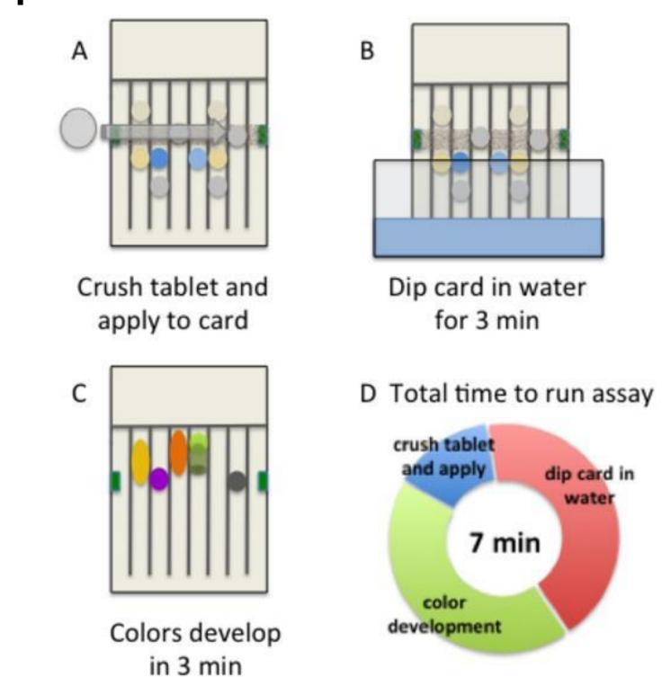
Chemical fingerprint: The chemical compounds present in the drug react with the reagents in the vertical lanes of the PAD. These reactions produce colors coming in contact with water and is unique for that drug.
